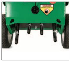
Four Tensile hardened thin wall tines Simple, durable screw in design makes service simple. In/out reciprocating tine motion produces less compaction on the inner surface of the hole compared to spoon designs.
