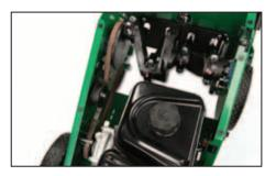
Longer belt span improves belt de-clutching and increases belt life.
